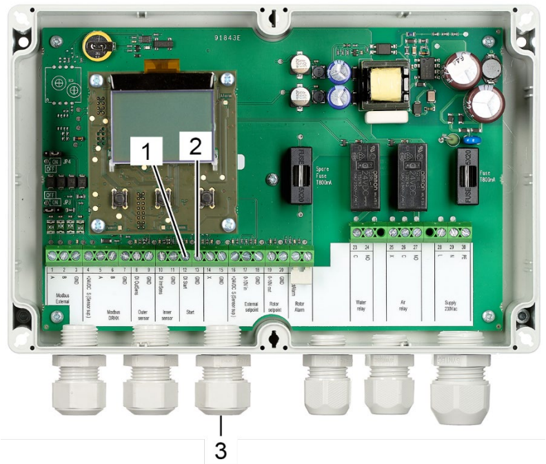
Fig. 92: Terminals external start signal
