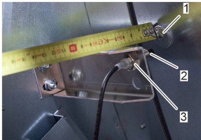
Fig. 77: Adjust clock sensor
