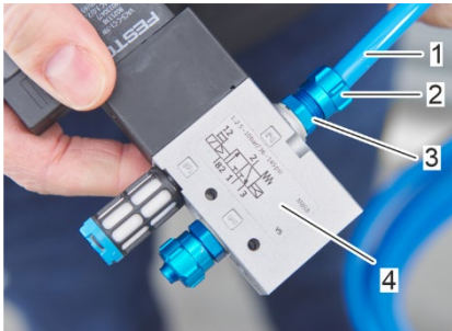
Fig. 65: Secure the compressed air hose on connection 2
