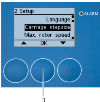
Fig. 127: Open submenu "carriage stepsize"
