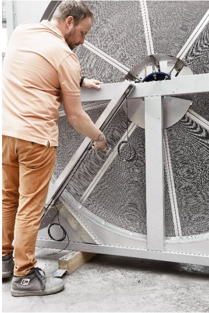
Fig. 47: Cleaning carriage middle position
