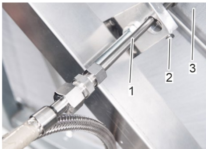
Fig. 42: Adjust the distance of the water nozzle to the rotor surface
