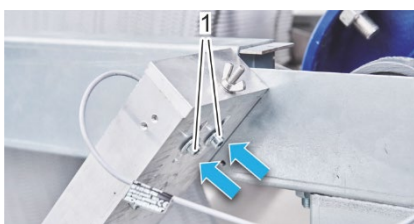
Fig. 32: Screws of the deflector roll
