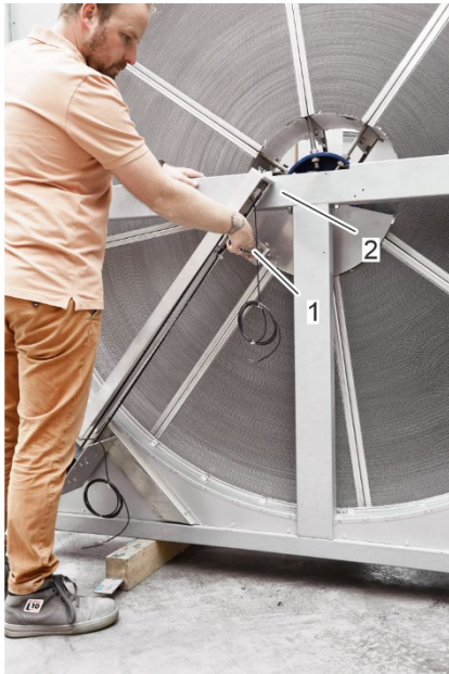
Fig. 36: Cleaning carriage top position
